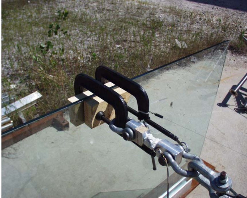
Fig. 3 - An overall view of the glass panel test setup is shown. The load was applied at the center of the top edge of the glass panel. Wood blocks were used to distribute the clamping pressure and prevent fracture of the glass.
