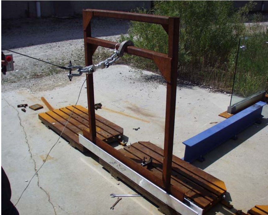
Fig. 1 - An overall view of the first test setup is shown. The load was applied at the center of the of the substitute steel rail.
